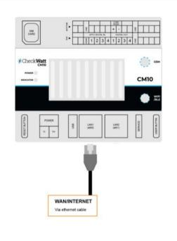
The **ethernet** cable needs to be **stripped** on **one side** where pin 4 (Blue) and pin 5 (blue/white) represent 485B and 485A, respectively.
