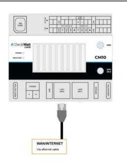
The **Ethernet cable** needs to be **stripped** on **one side** where pin 1 represents 485\_B and pin 2 represents 485\_A.
